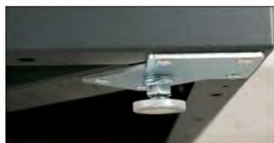
Adjustable feet from the inside.
